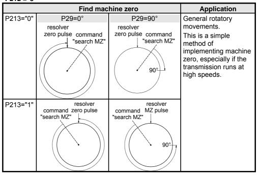
Machine zero equals external initiator (without resolver zero)
